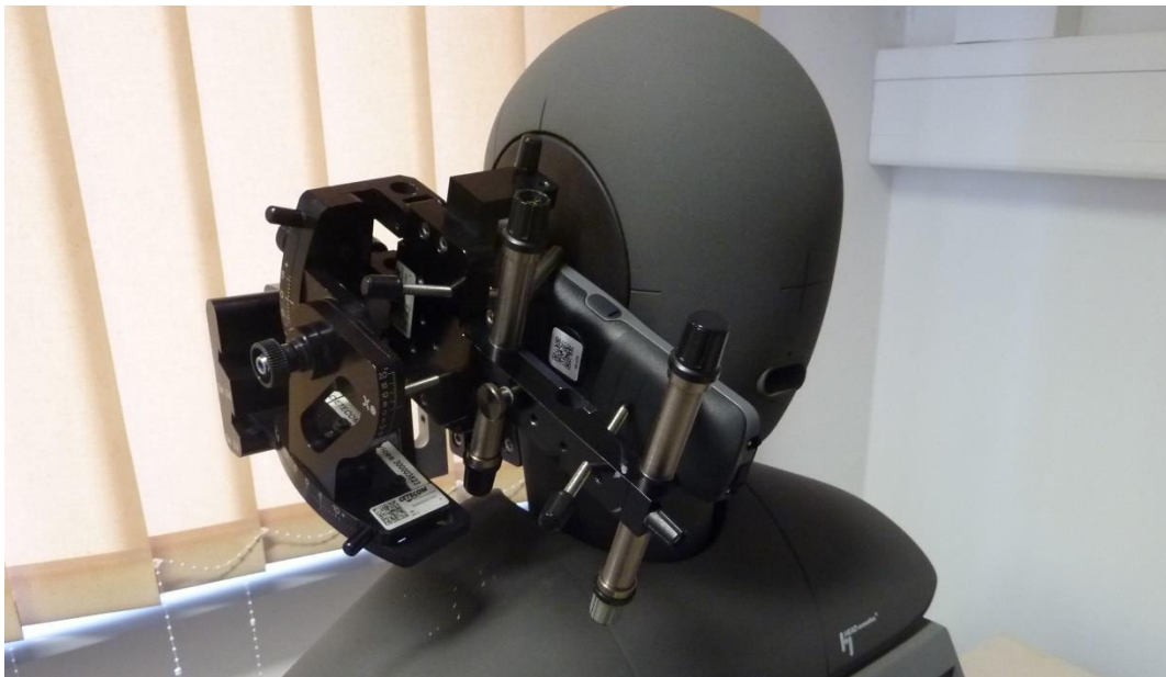
Photo 2: test setup for volume control (close-up view)
