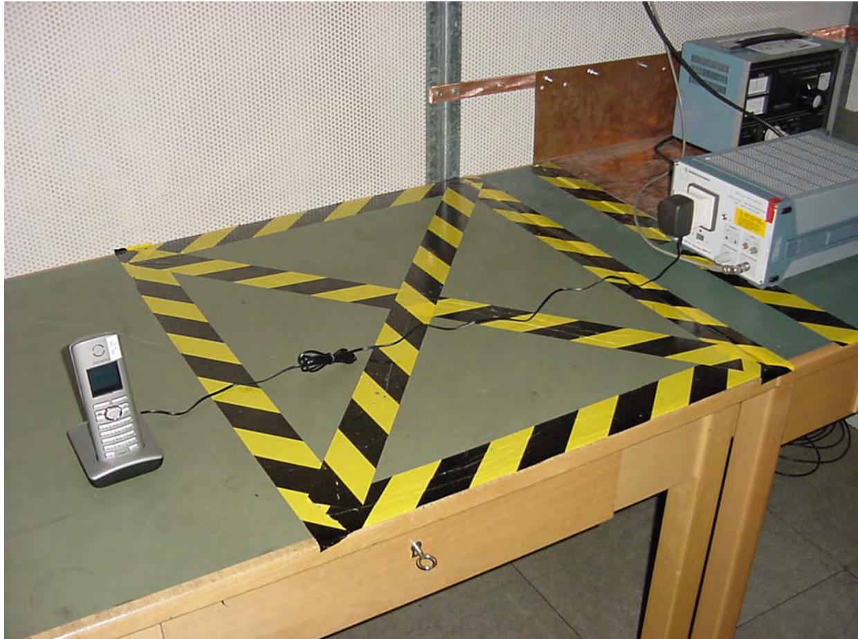
Photo 3: Conducted Emissions S45
