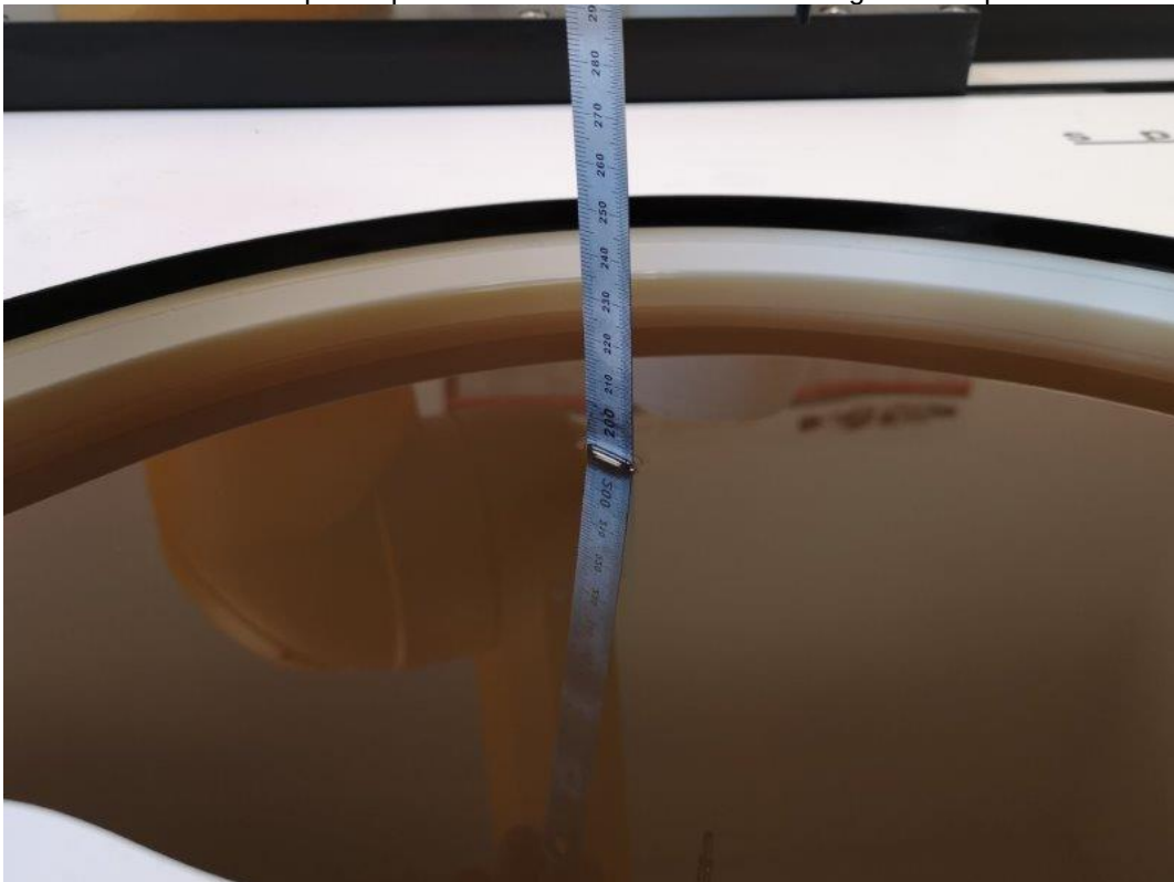
Photo 2: Liquid depth HBBL600-10000MHz Simulating Head Liquid
