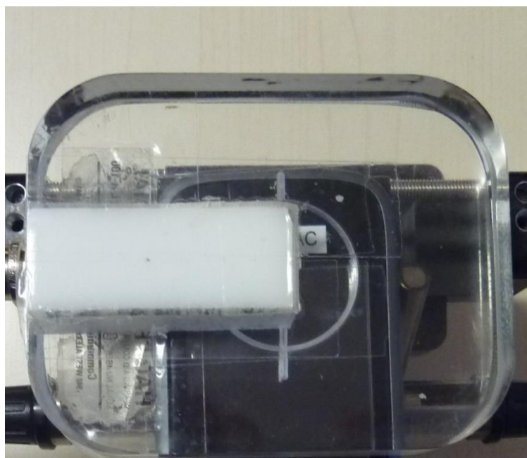
Photo 4: test setup for Radial field intensity (0 degree)
