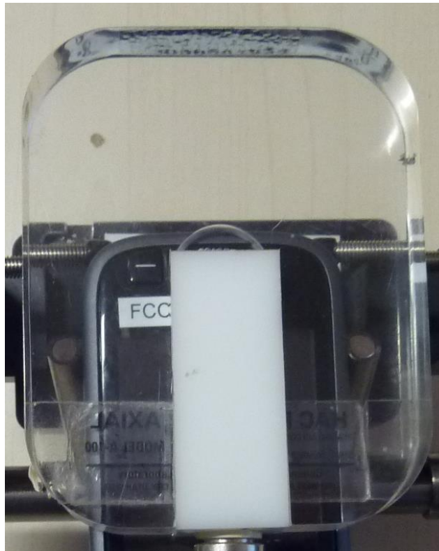
Photo 3: test setup for axial field intensity and magnetic field intensity frequency response
