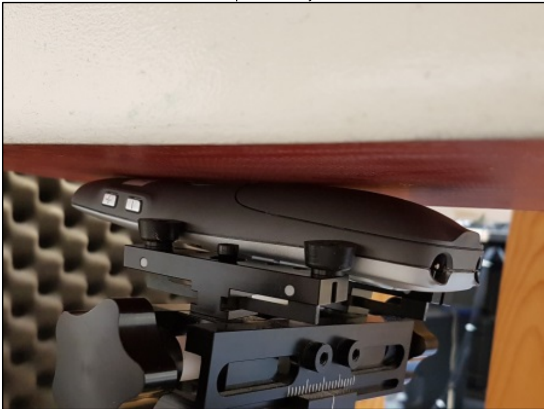
Photo 19: Test position body worn rear side
