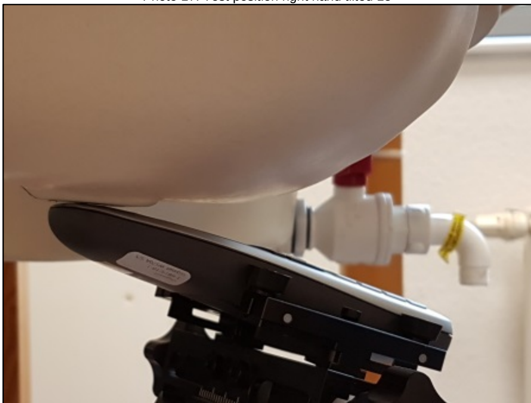
Photo 18: Test position body worn front side
