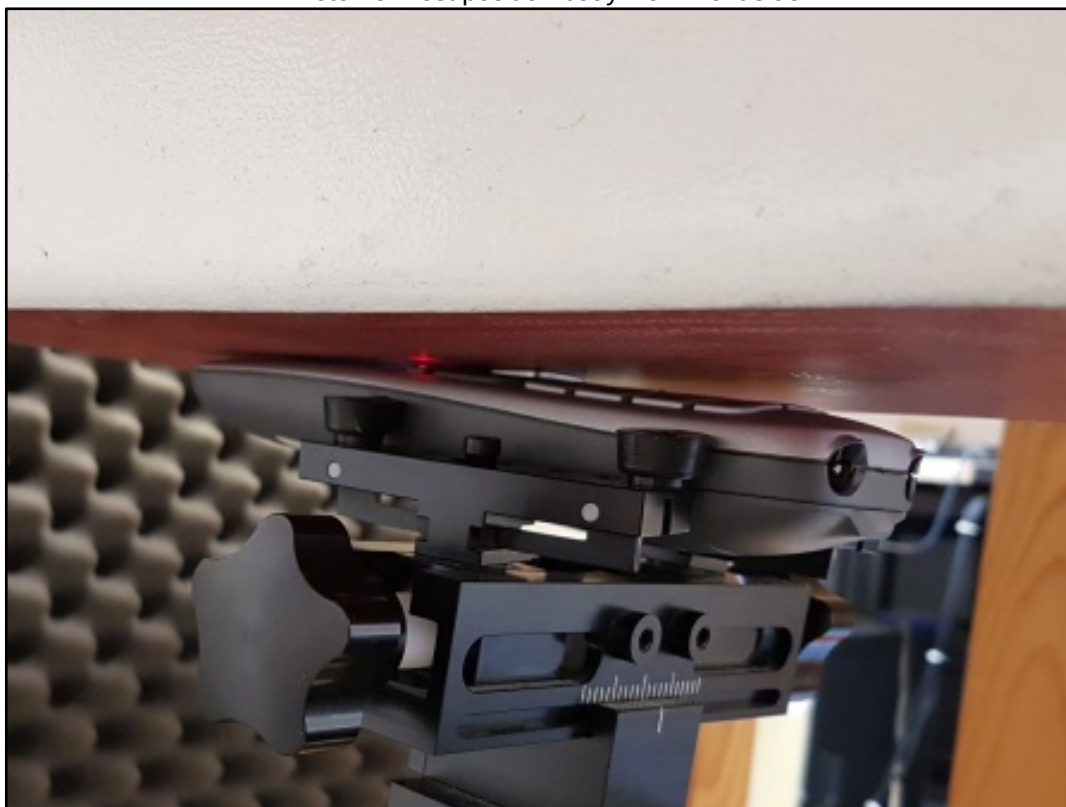
Photo 18: Test position body worn front side
