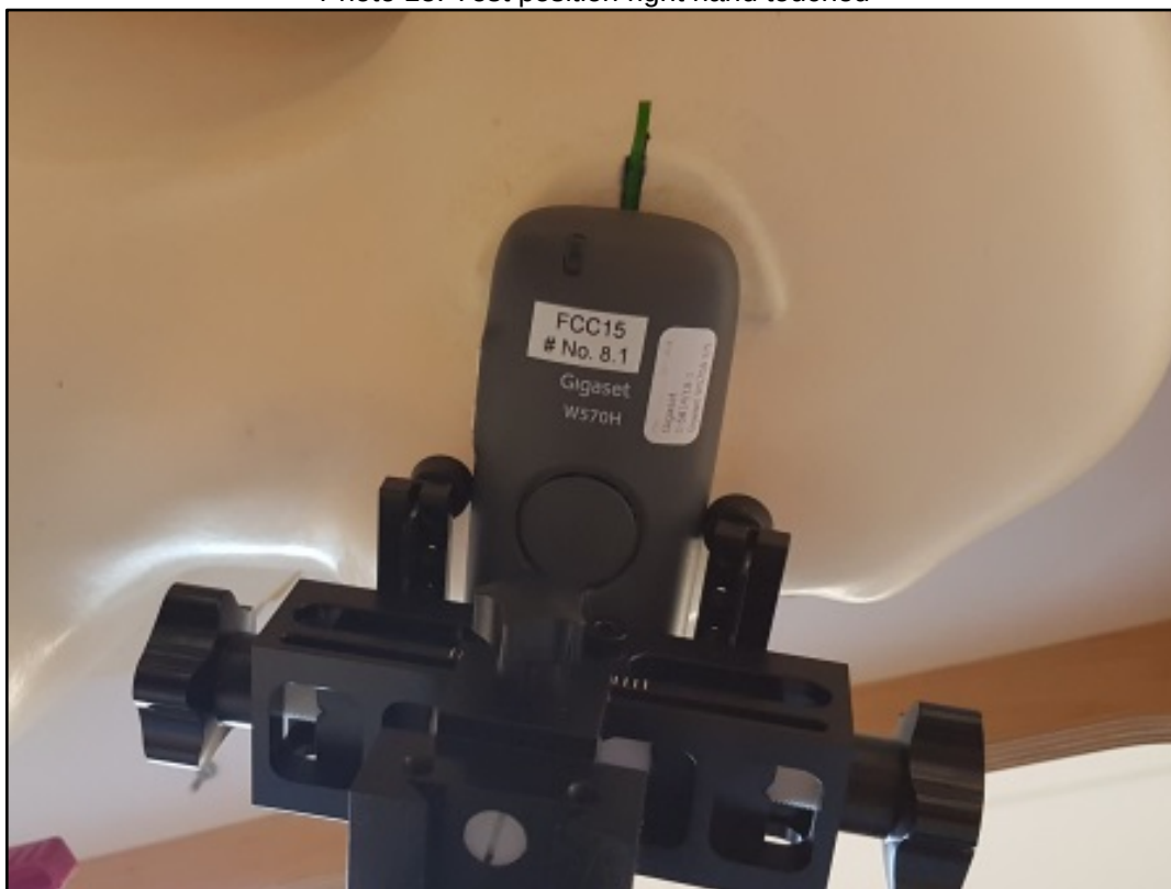
Photo 16: Test position right hand tilted 15°
