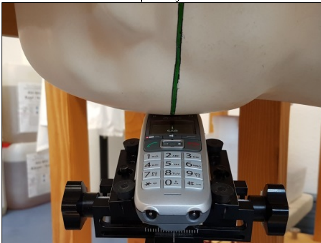
Photo 16: Test position right hand tilted 15°
