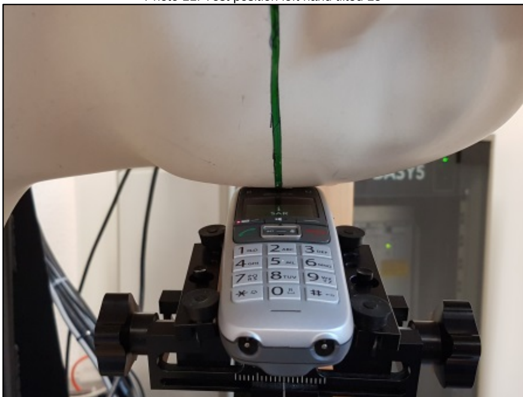
Photo 12: Test position left hand tilted 15°
