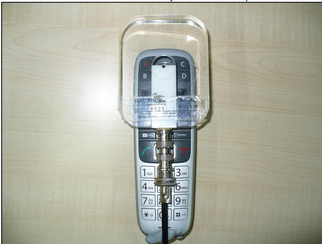
Photo 4: Radial field intensity measurement set-up (0 degree)
