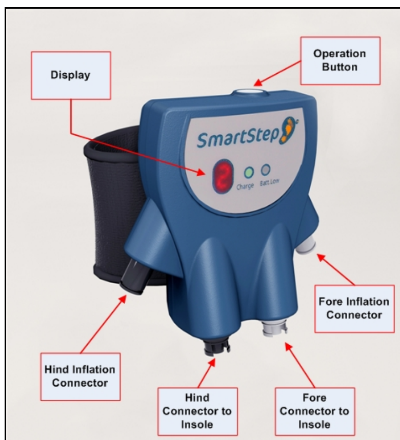
The Control Unit
