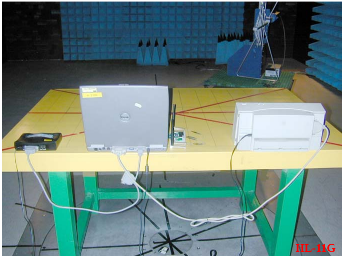
Photo 2: Radiated Emission Test Set-up
