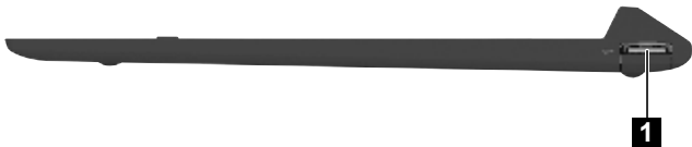
1 USB 2.0 port Connects to USB 2.0 devices.
