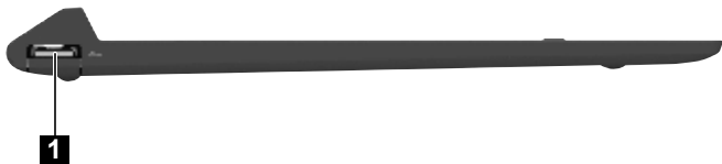
1 USB 2.0 port Connects to USB 2.0 devices.
