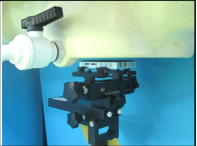
Rear Face of EUT with 0.5 cm Gap
