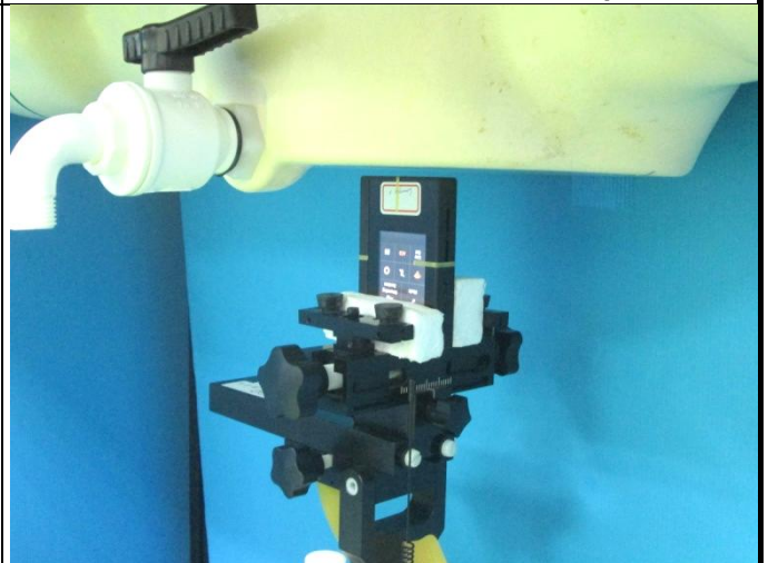
Bottom Side of EUT with 0.5 cm Gap
