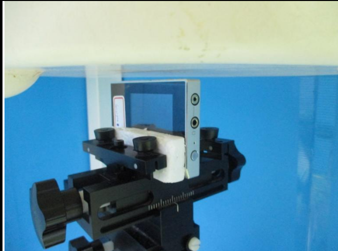
Left Side of EUT with 0.5 cm Gap
