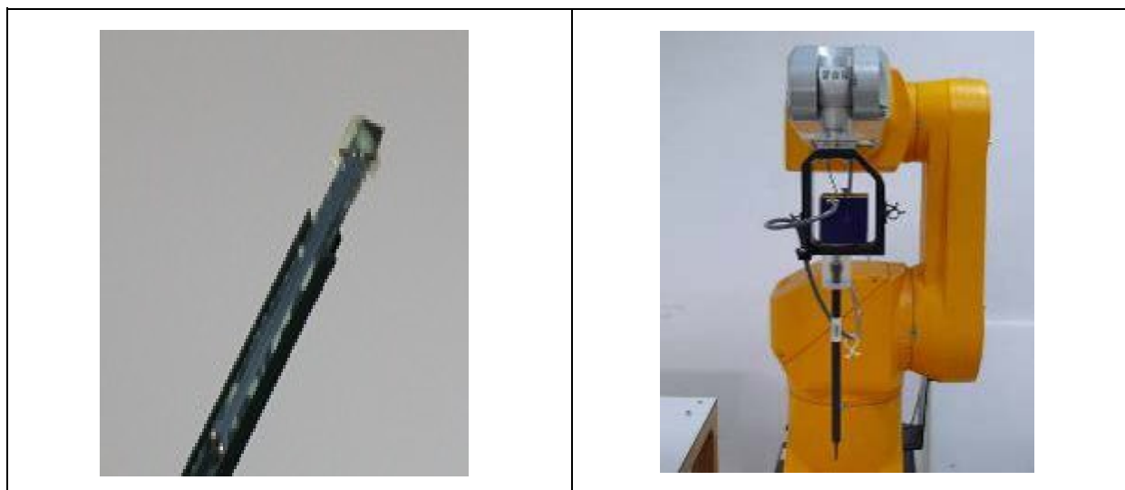
EX3DV4 E-field Probe
