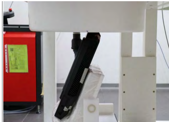
Fig.13 EUT position(2-8) to flat phantom
