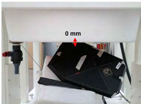
Fig.4 EUT position(1-2) to flat phantom
