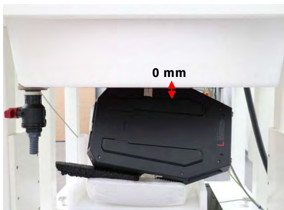
Fig.11 EUT position(2-6) to flat phantom
