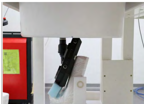
Fig.5 EUT position(1-4) to flat phantom
