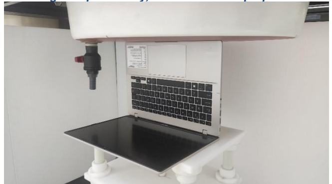
Testing Setup for Body, Front Side of Laptop at 0 mm
