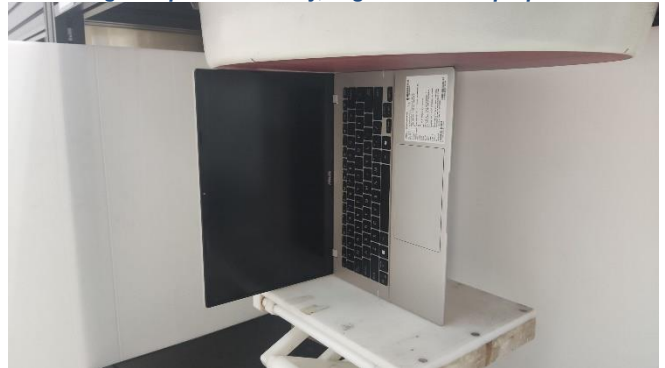
Testing Setup for Extremity, Right Side of Laptop at 0 mm
