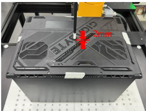
Photograph 3. PD, Bottom Surface, 2mm
