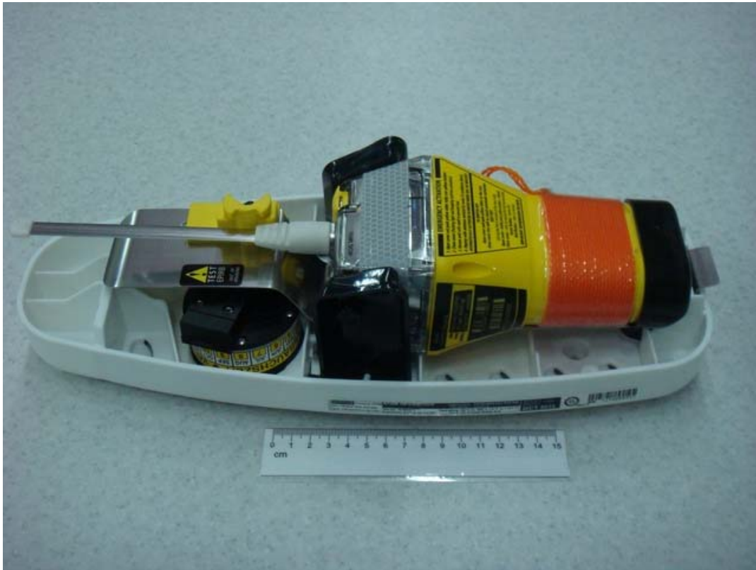
Figure 3.1 – General view of MT603FG (s/n 1410407582).
