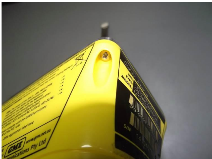
Figure 28.2 — Positions of 4 top screws
