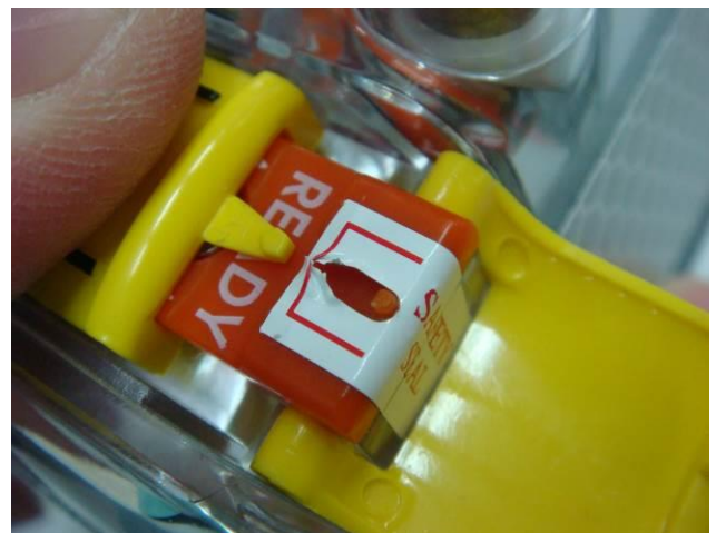
Figure 29.1 – Protecting EPIRB means which breaking indicates that the satellite EPIRB has been previously activated
