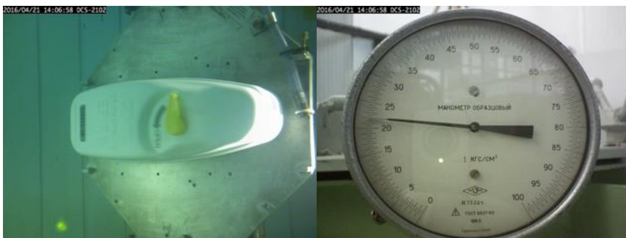
Figure 30.5 - The satellite EPIRB automatically released at Rolling 90° port orientation
