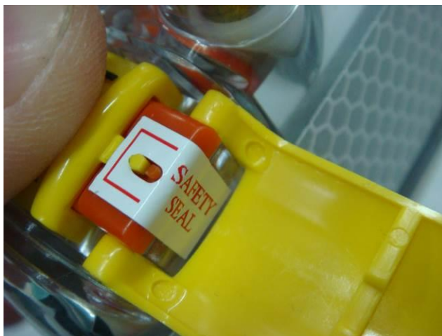
Figure 29.1 – Protecting EPIRB means which breaking indicates that the satellite EPIRB has been previously activated
