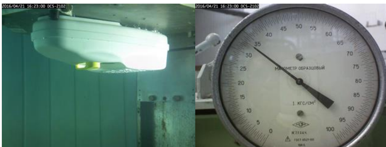
Figure 30.6 - The satellite EPIRB automatically released at Pitching 90° bow down orientation
