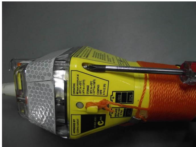
Figure 28.3- Remove the 4 top screws using a PZ1 screwdriver
