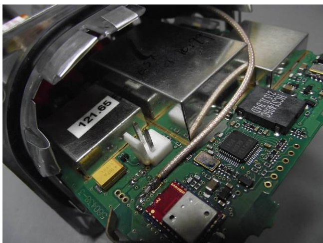
Figure 28.4- Remove the lid assembly by lifting it vertically away from the main body
