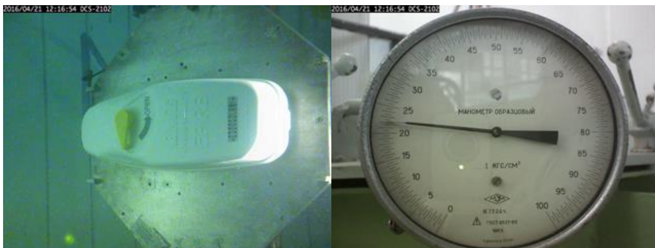
Figure 30.4 - The satellite EPIRB automatically released at Rolling 90° starboard orientation
