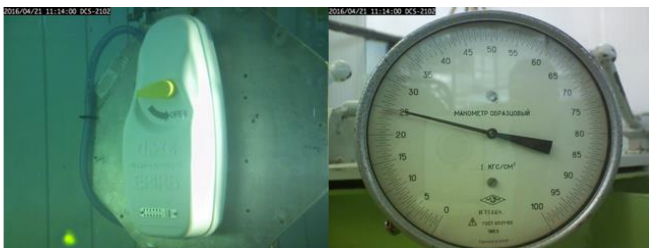
Figure 30.3 - The satellite EPIRB automatically released at normal orientation at ambient temperature
