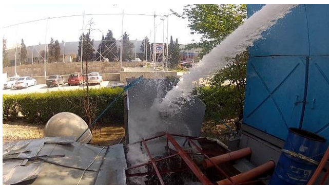
Figure 17.6 - The water strikes EUT (MT603FG) in an arc of 180°.
