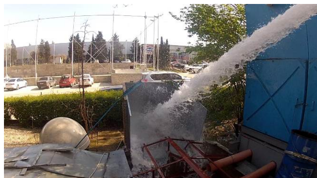
Figure 17.6 - The water strikes EUT (MT603FG) in an arc of 180°.
