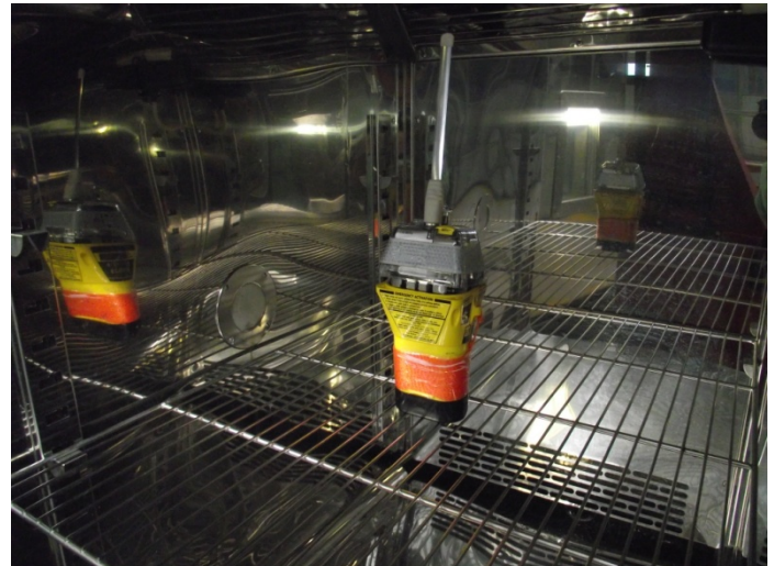
Figure 19.2 - View of the modified MT603FG installed in climatic chamber
