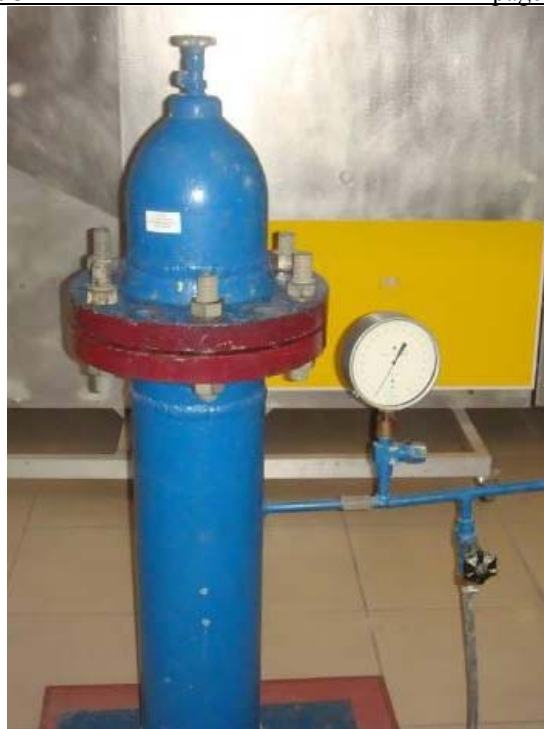
Figure 9.2 – View of immersion test site (Manometer of immersion test site indicates 1 bar)
