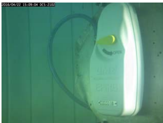
Figure 15.2 - The satellite EPIRB automatically released at normal orientation after maintained at maximum storage temperature.
