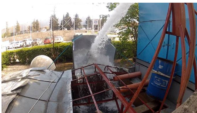
Figure 17.5 - The water strikes EUT (MT603G) in an arc of 180°.
