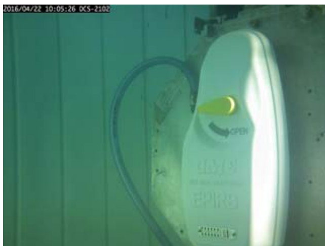
Figure 15.1 – The satellite EPIRB automatically released at normal orientation after maintained at minimum storage temperature.
