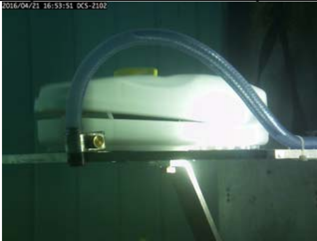
Figure 15.7 - The satellite EPIRB automatically released at Pitching 90° stern down orientation
