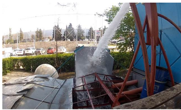
Figure 17.5 - The water strikes EUT (MT603G) in an arc of 180°.
