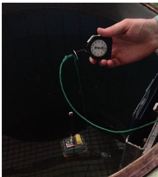
Figure 16.3 – Measuring of buoyant force
