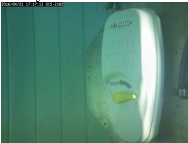
Figure 15.8 - The satellite EPIRB automatically released at Upside down orientation
