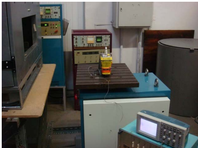
Figure 5.2 - Test Set-up. Vertical axis of the MT603G
