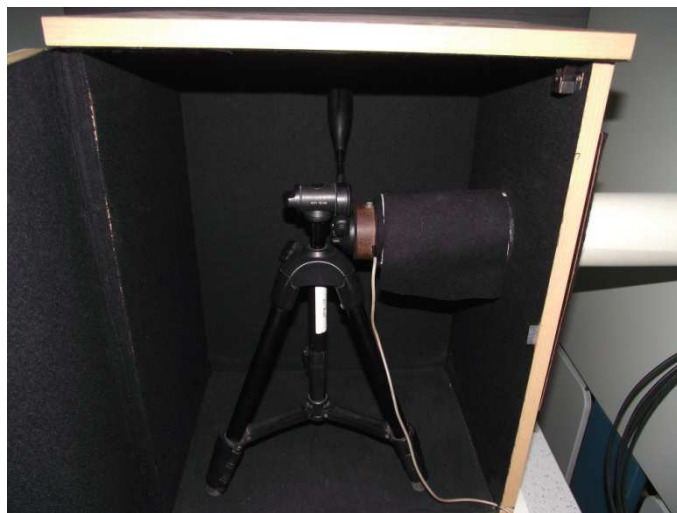
Figure 13.2 – General view of graphic luxmeter
