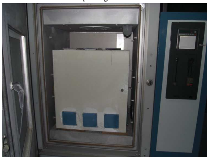
Figure 13.3 – General view of rotation and inclination device inside of the climatic chamber
