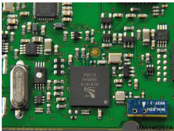
XWP – BT Transceiver + Antenna (FMX PBA)
