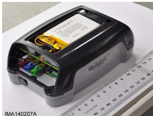
Internal Battery Location
