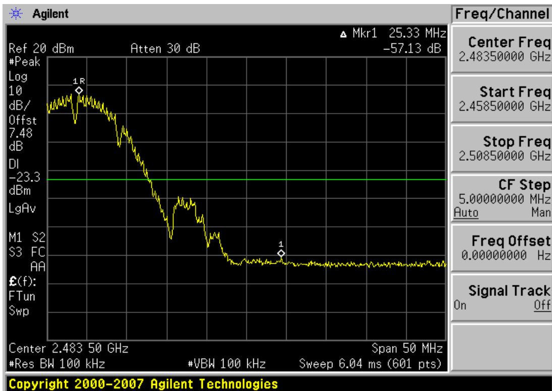
Plot 6-20. Band Edge Plot (802.11b – Ch. 11)
