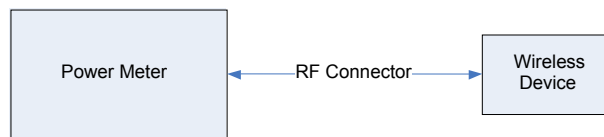
Figure 12-1 Power Measurement Setup
