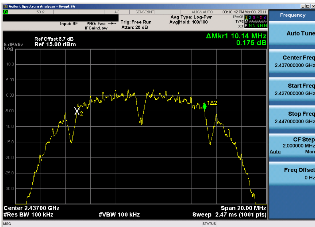
Plot 6-2. 6dB Bandwidth Plot (802.11b - Ch. 6)
