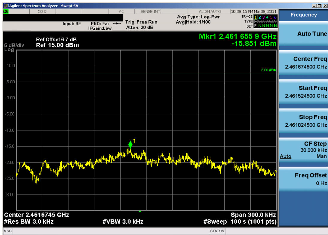
Plot 6-18. Power Spectral Density Plot (802.11n – Ch. 11)
