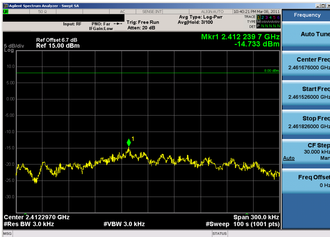
Plot 6-16. Power Spectral Density Plot (802.11n – Ch. 1)
