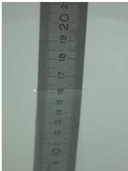
Fig. 19: Liquid depth for 2450 MHz Body measurements.
