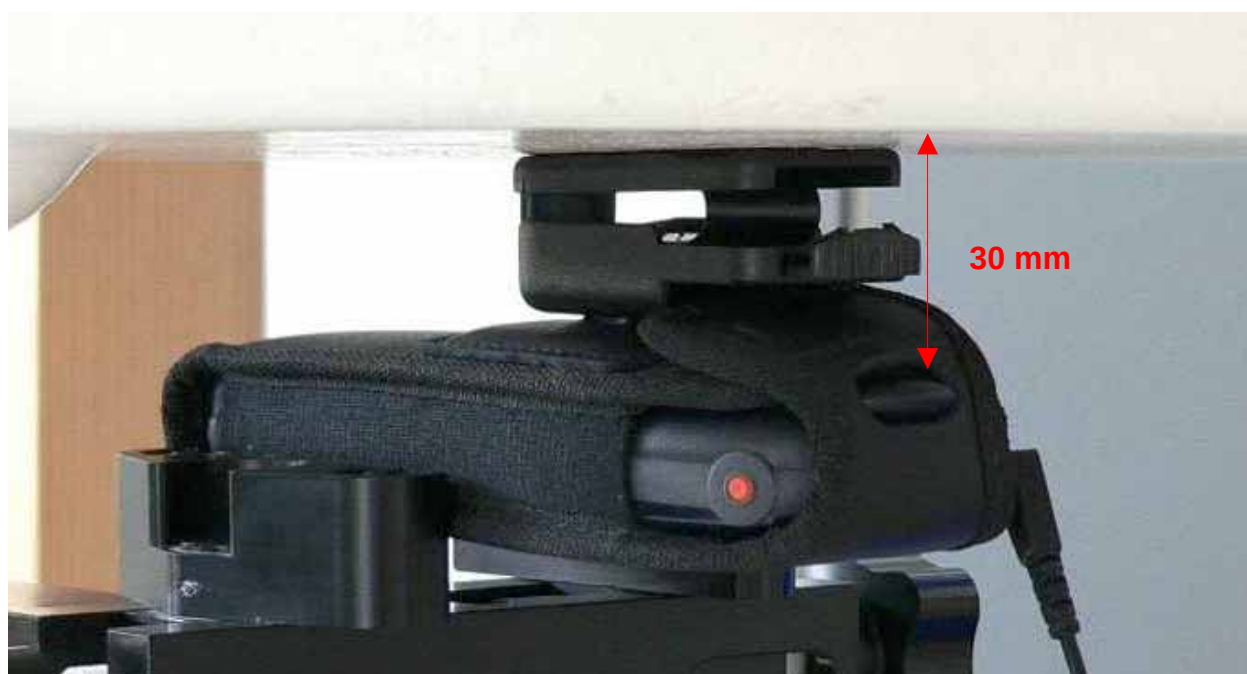
Fig. 18: Picture of the device tested with leather case, rotation clip and headset.
