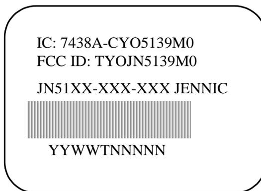
Figure 9: Example module labelling for FCC approved modules
