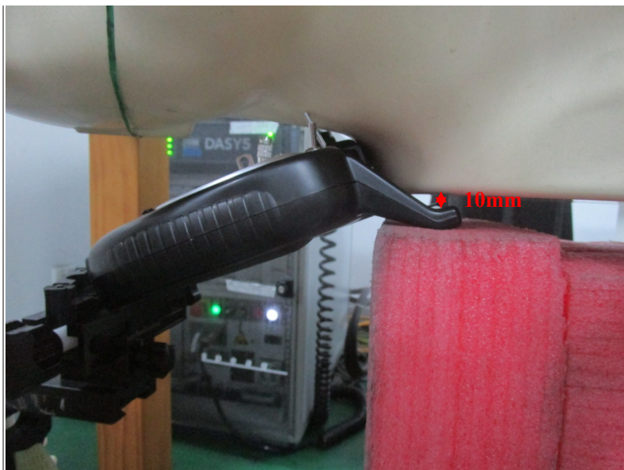
Close to Body Front Setup Photo(10mm)
