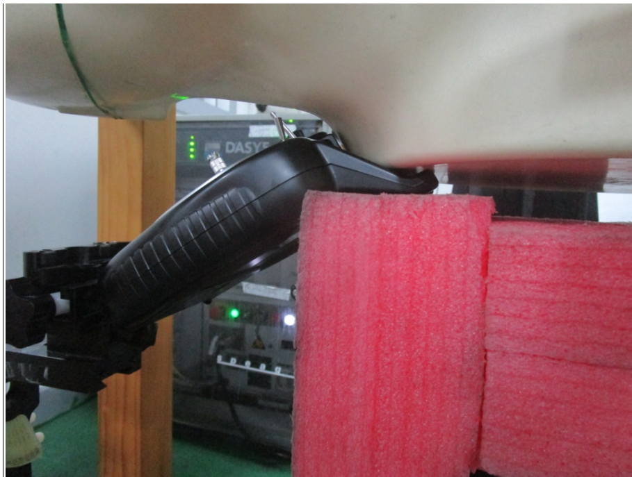
Handheld Front Setup Photo(0mm)
