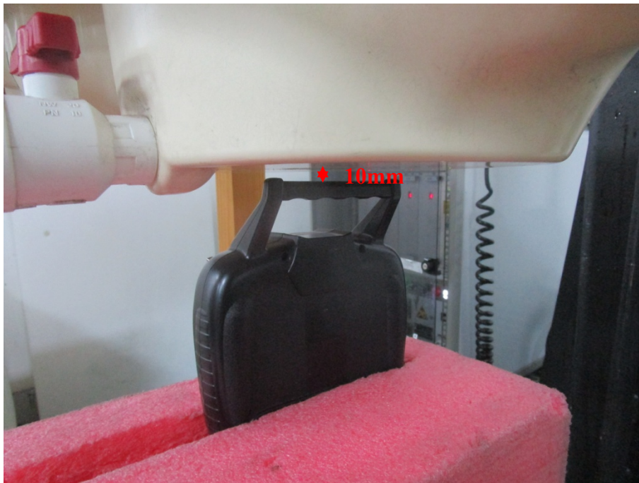
Close to Body Top Setup Photo(10mm)
