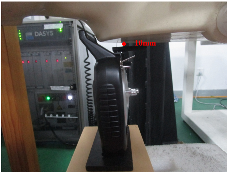
Close to Body Top Setup Photo(10mm)
