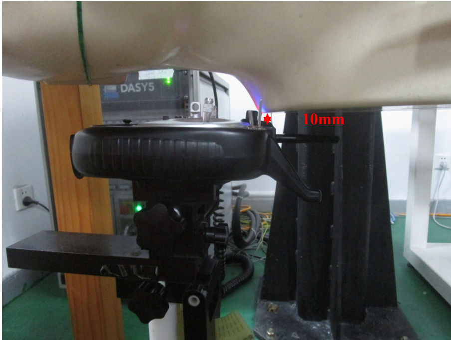
Close to Body Front Setup Photo(10mm)
