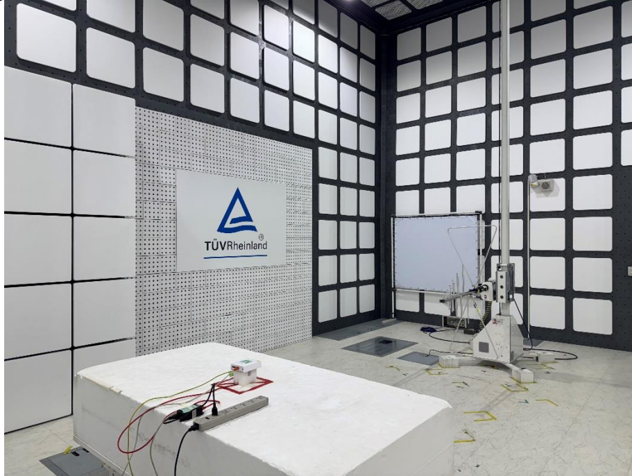
Photograph 11: Test Setup for Spurious Emissions (Back View 2)
