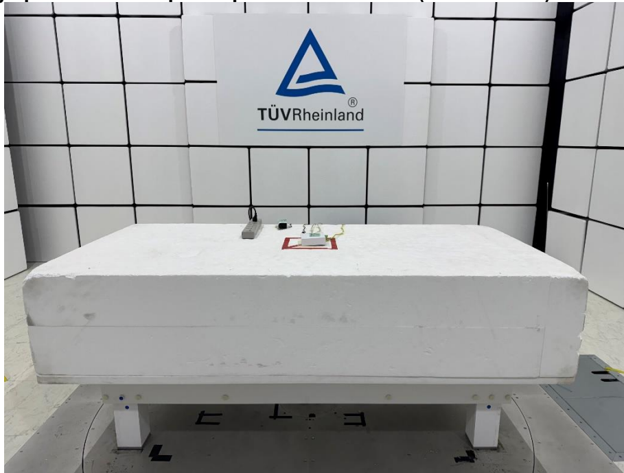
Photograph 2: Test Setup for Spurious Emissions (Front View 2)
