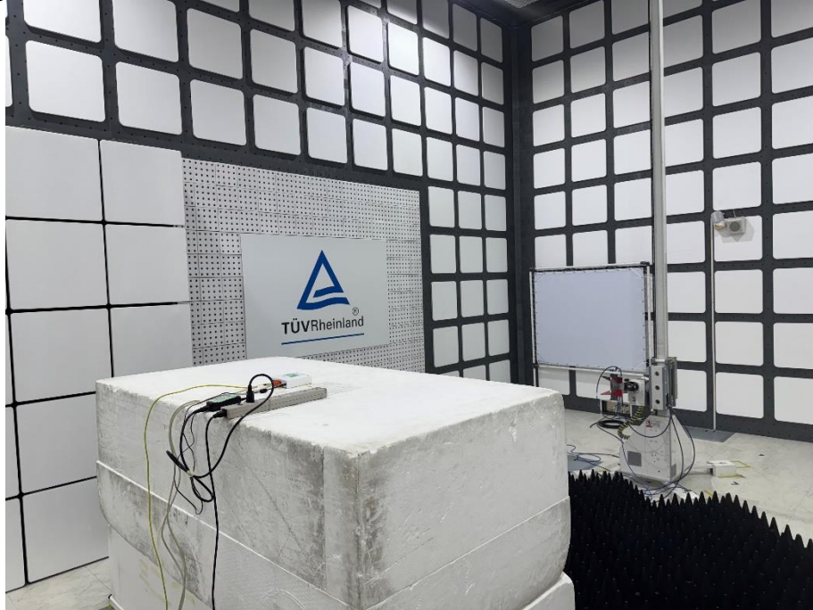
Photograph 5: Test Setup for Spurious Emissions (Back View 3)
