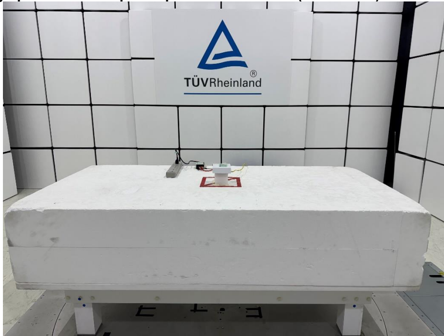
Photograph 10: Test Setup for Spurious Emissions (Back View 1)
