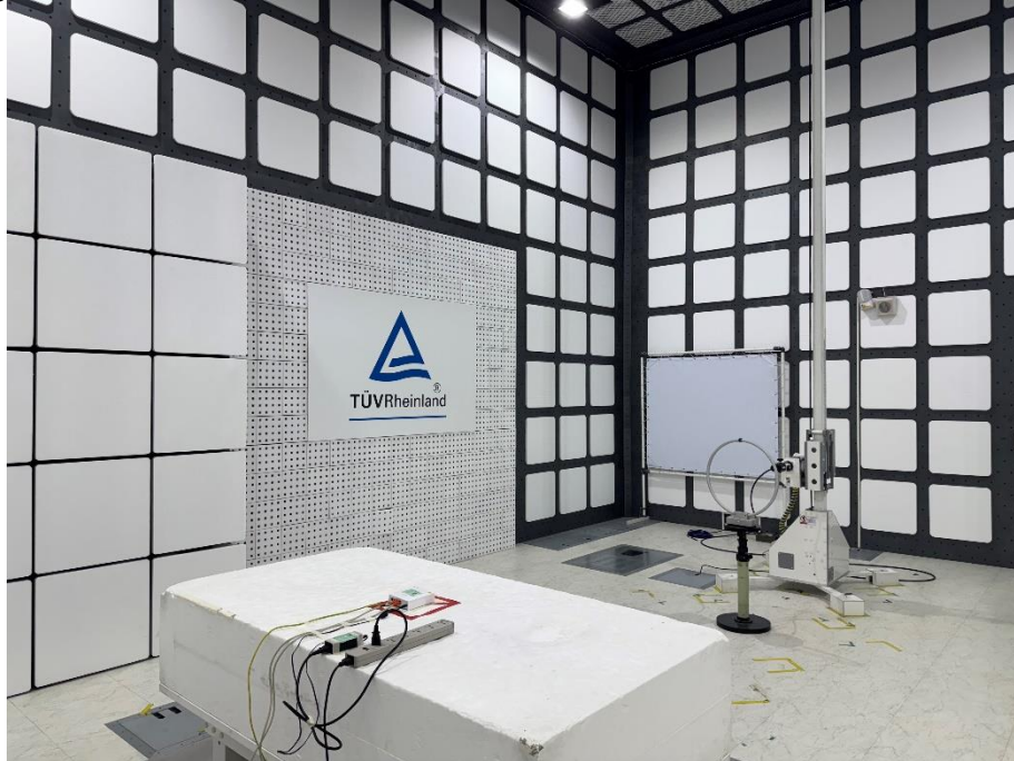
Photograph 3: Test Setup for Spurious Emissions (Back View 1)
