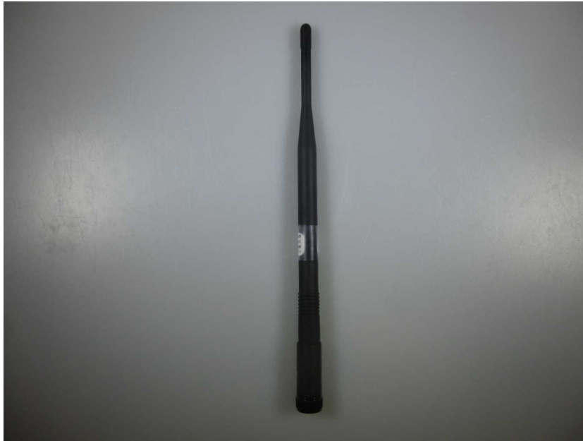
Photo 9: External dipole antenna
