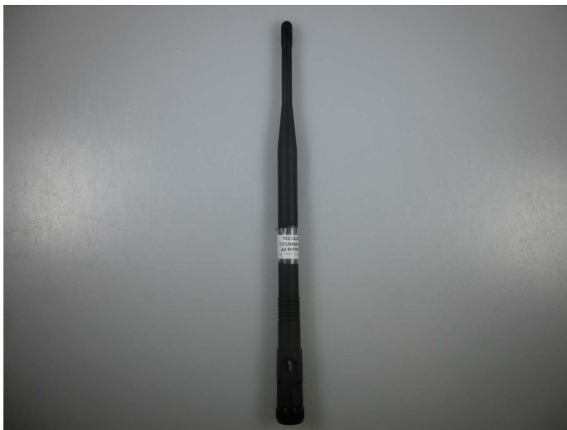
Photo 10: External dipole antenna
