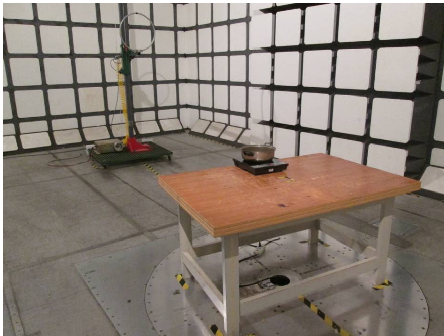
Radiated Emissions - Front View (Below 30MHz)
