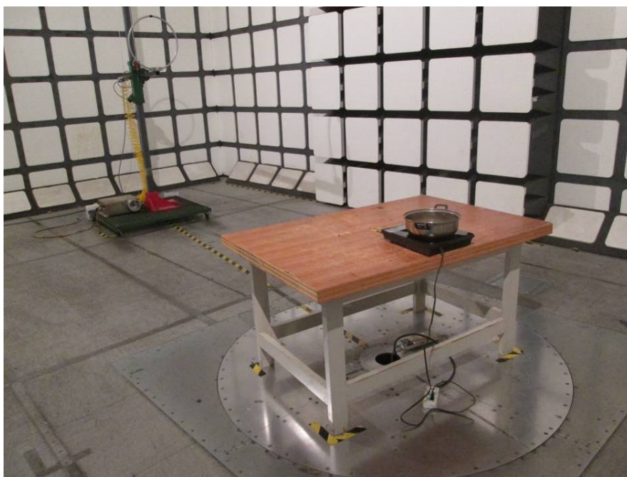
Radiated Emissions - Rear View (Below 30MHz)
