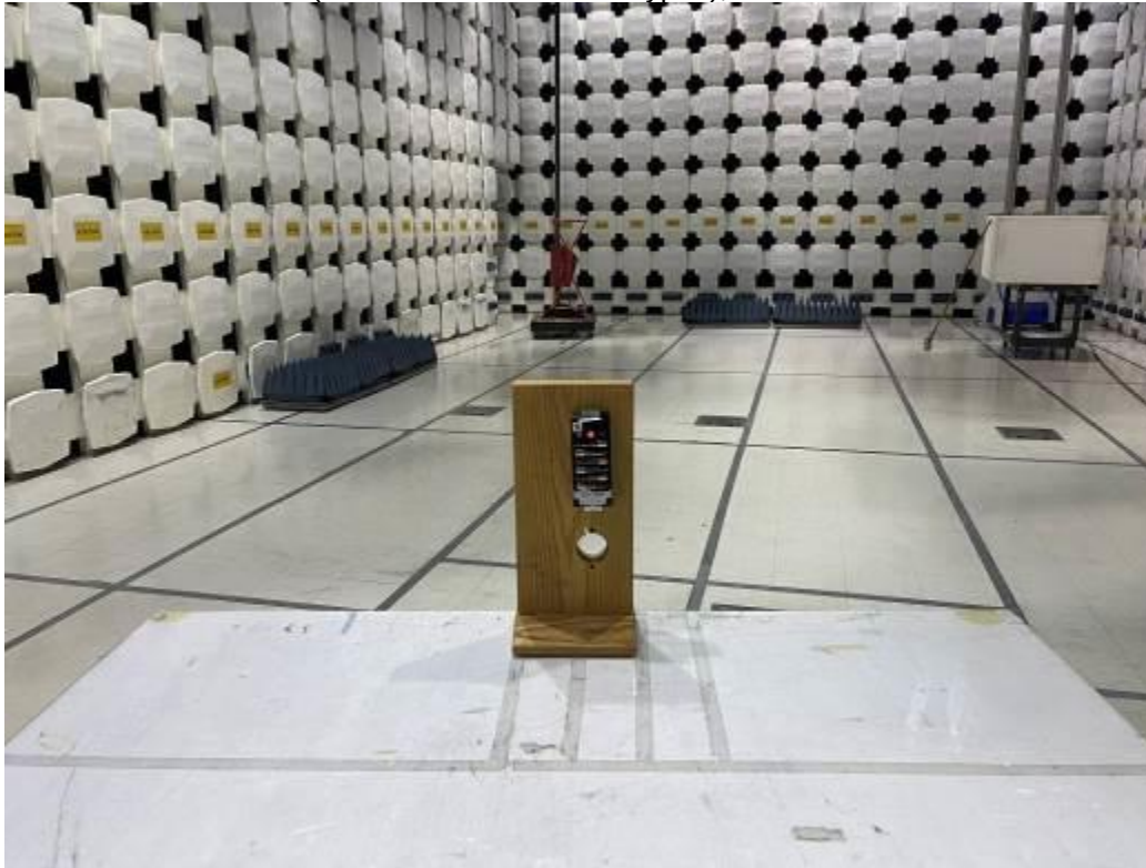
BLE (Metal Enclosure With Keypad), 30-1000 MHz
