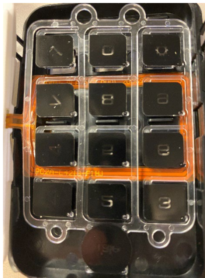
RFID Antenna Behind Push Buttons
