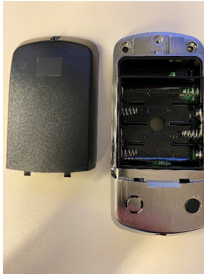
Front with Battery Cover Removed
