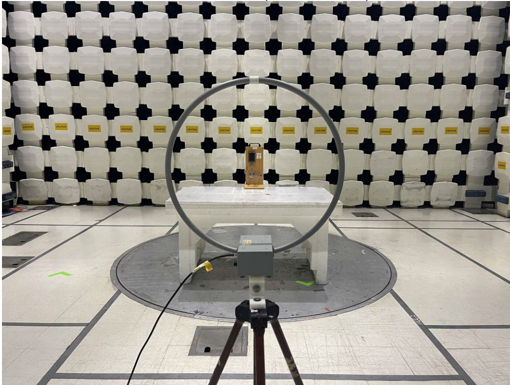
NTM613-ACC Push Button (13.56 MHz RFID), X-axis
