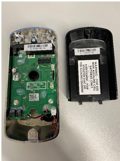
Back with backplate removed
