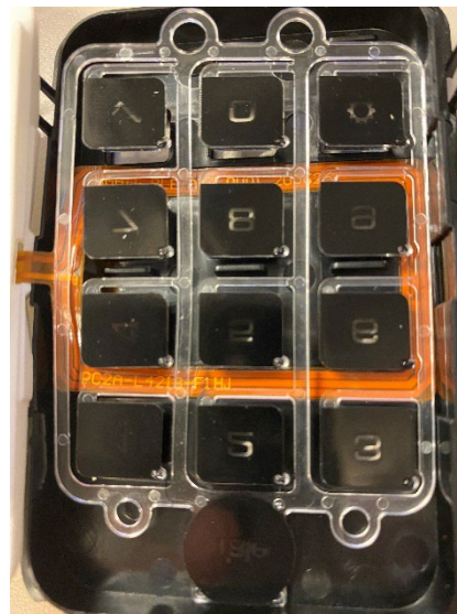
RFID Antenna Behind Push Buttons
