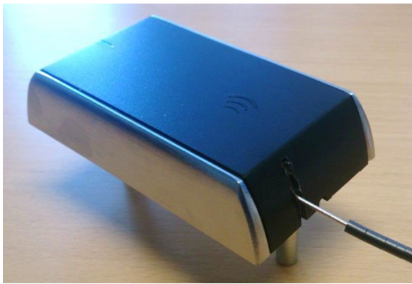
Fig 1: IN100 plastic cover with metal wings.
