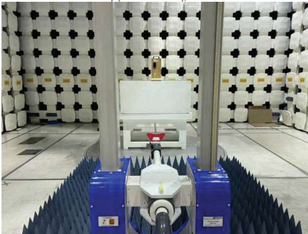
Test Setup (Plastic Enclosure), RE 1-18 GHz
