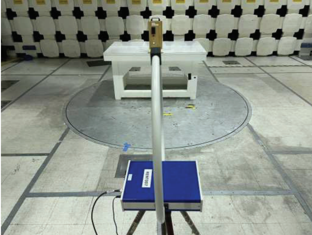
125 kHz and 13.56 MHz RFID (Plastic Enclosure) Test Setup, Z-axis, RE 9 kHz-30 MHz
