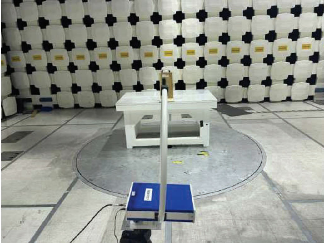
125 kHz and 13.56 MHz RFID (Metal Enclosure) Test Setup, Z-axis, RE 9 kHz-30 MHz
