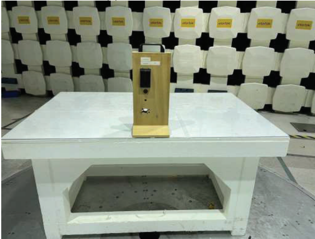
Test Setup (Plastic Enclosure), RE 30-1000 MHz
