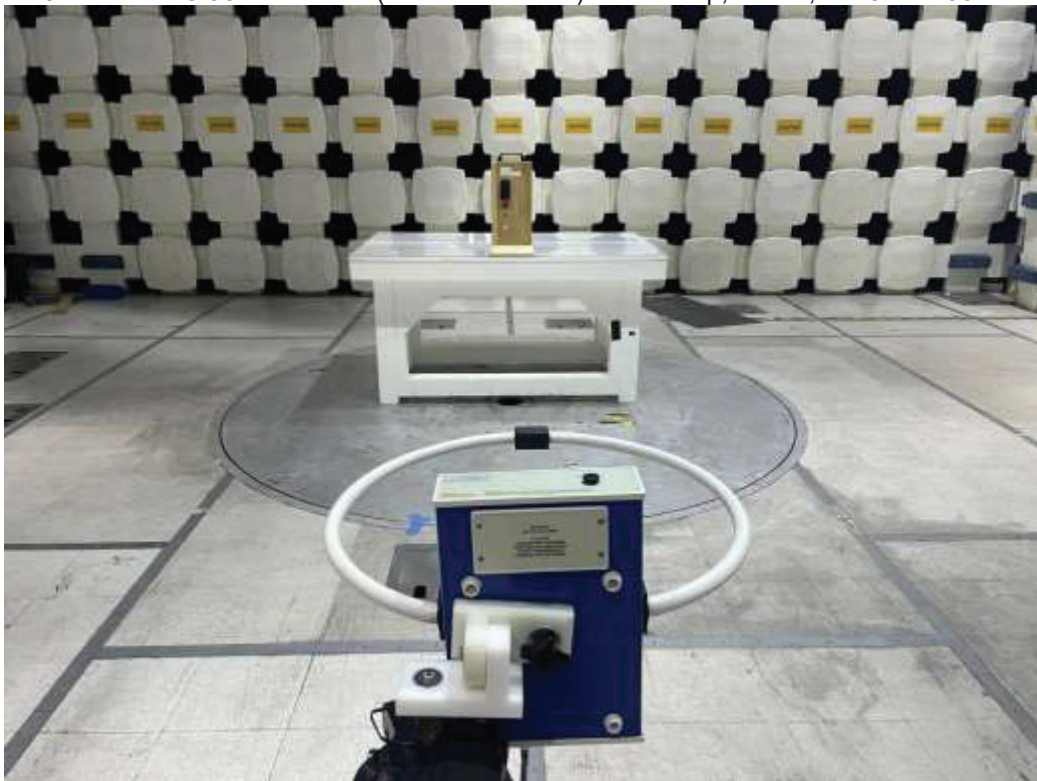
125 kHz and 13.56 MHz RFID (Metal Enclosure) Test Setup, Z-axis, RE 9 kHz-30 MHz
