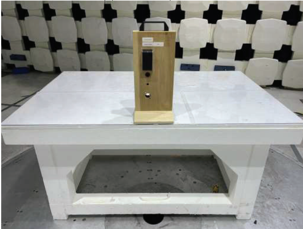
Test Setup (Metal Enclosure), RE 30-1000 MHz
