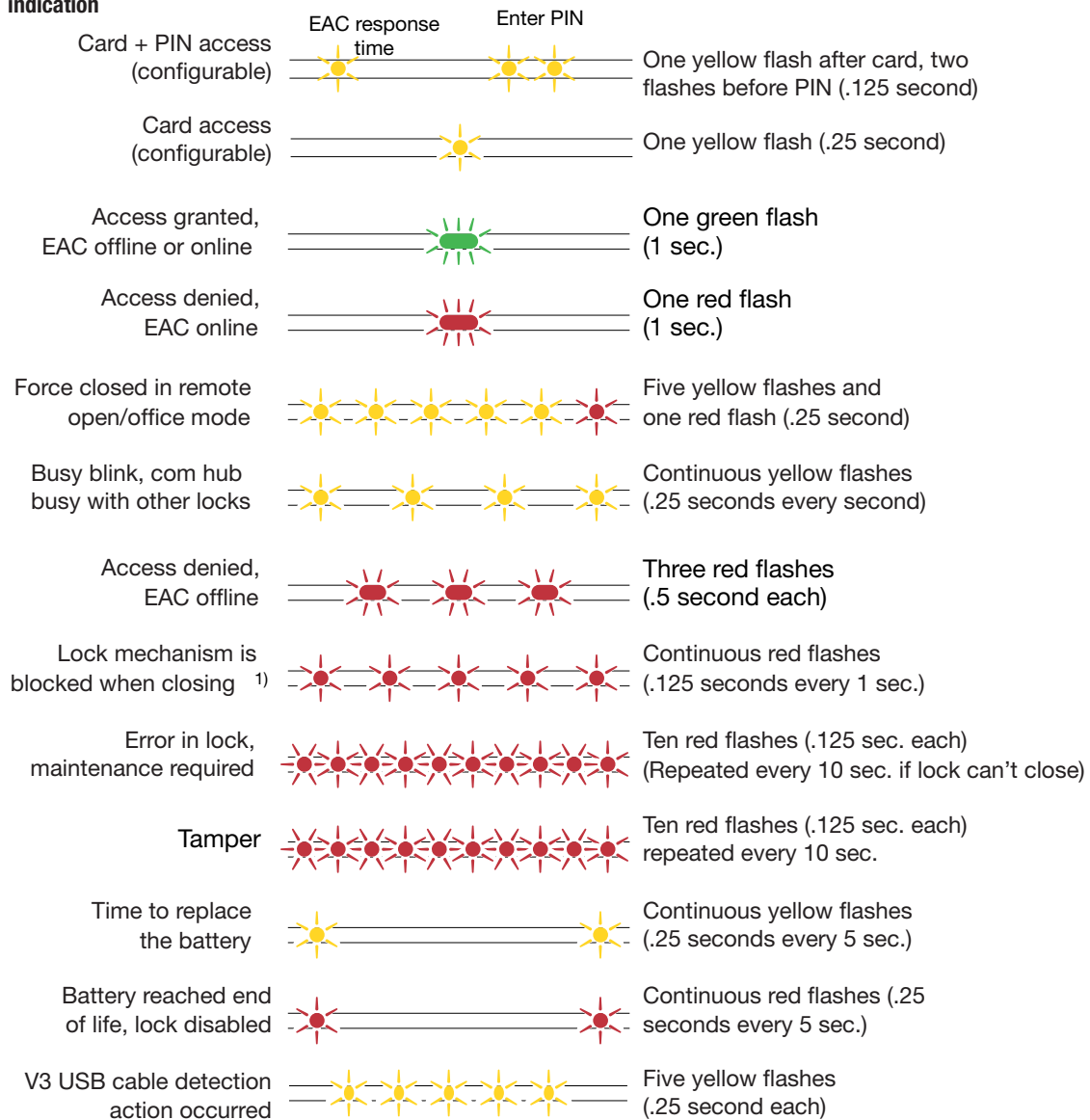
Figure 4. Lock normal operation LED indication
