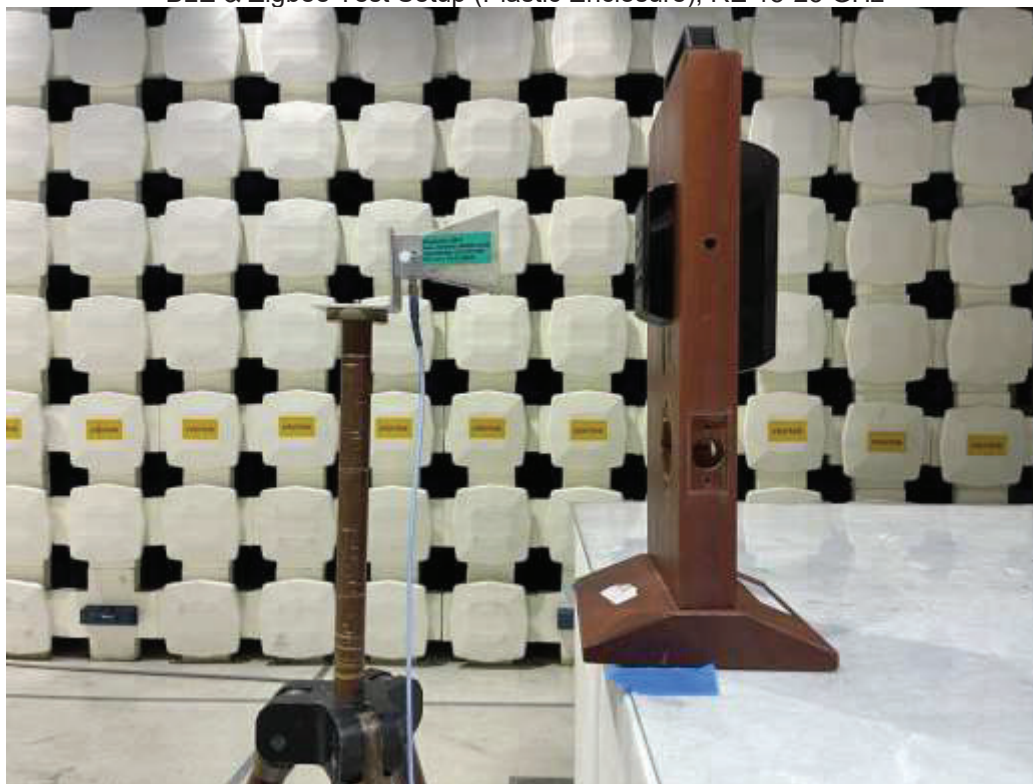
BLE &amp; Zigbee Test Setup (Plastic Enclosure), RE 18-25 GHz
