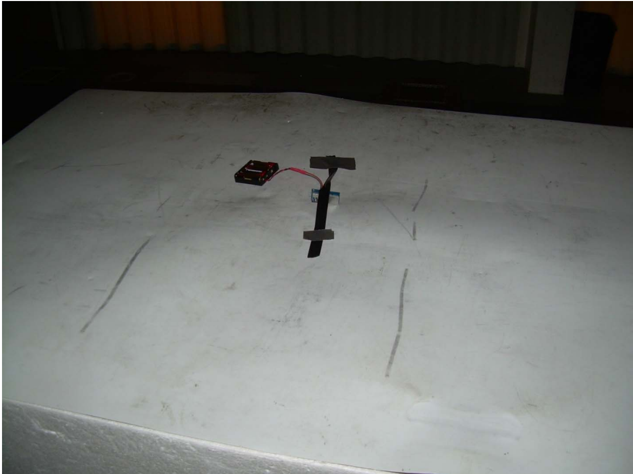
Photograph 3 – Front View of the Radiated Emission Setup – Vertical On-Edge on Table
