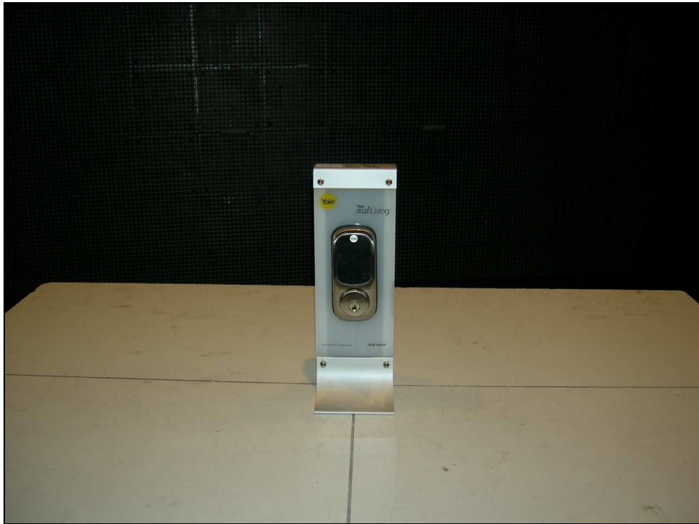
Figure 1: Radiated Emissions – Touchscreen Deadbolt – YRD220
