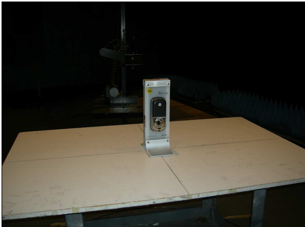
Figure 2: Radiated Emissions – Touchscreen Deadbolt – YRD220
