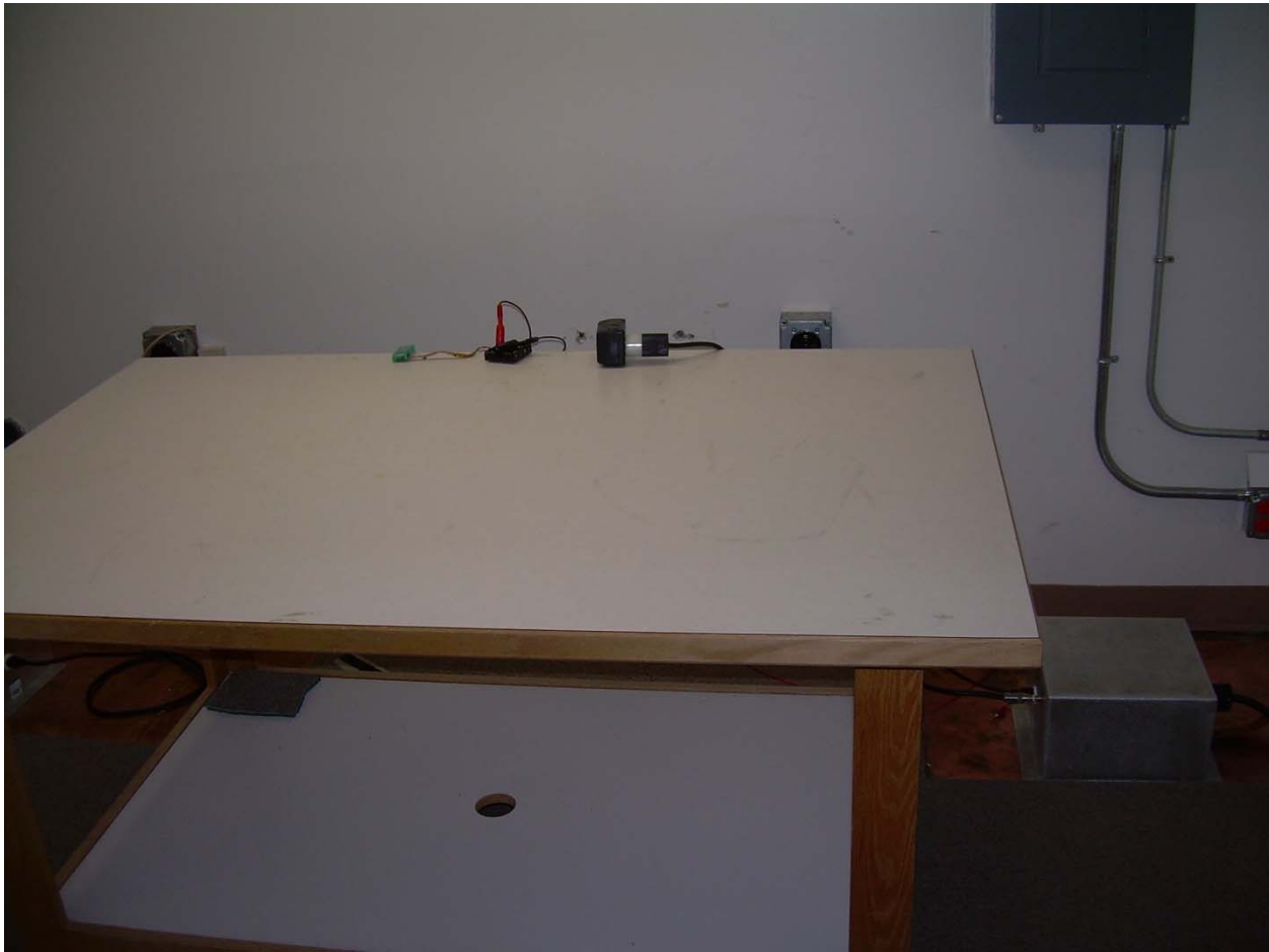
Photograph 5 – Front View Conducted Disturbance Worst Case Configuration
