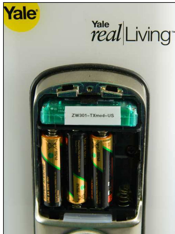
Figure 7: External Photo – EUT installed in host
