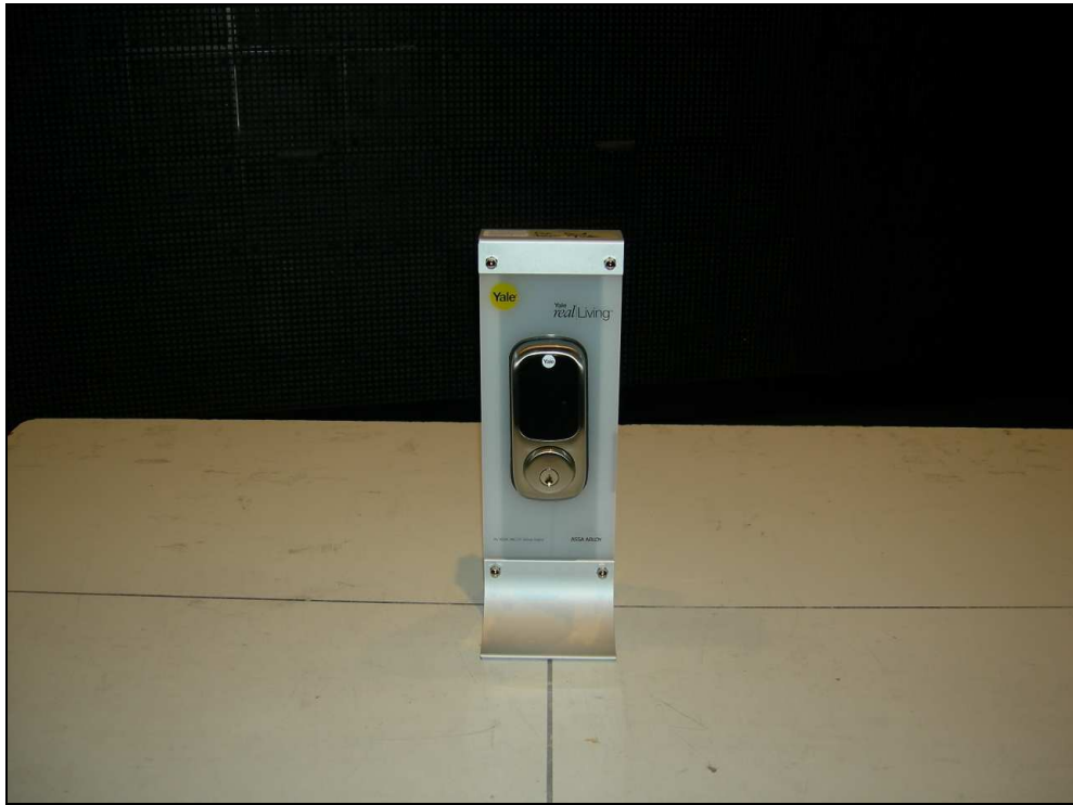
Figure 3: Radiated Emissions – Touch Screen Deadbolt Lock
