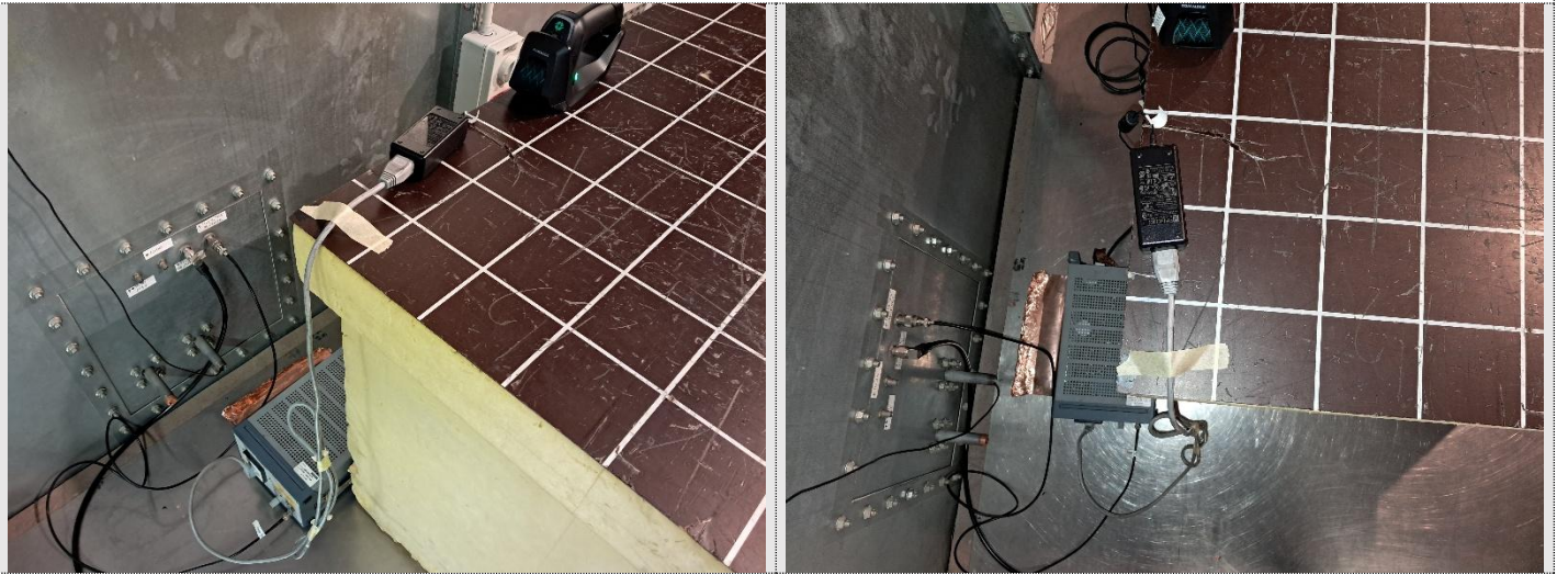
PHOTO N° 5 - CONDUCTED EMISSION TEST SETUP
