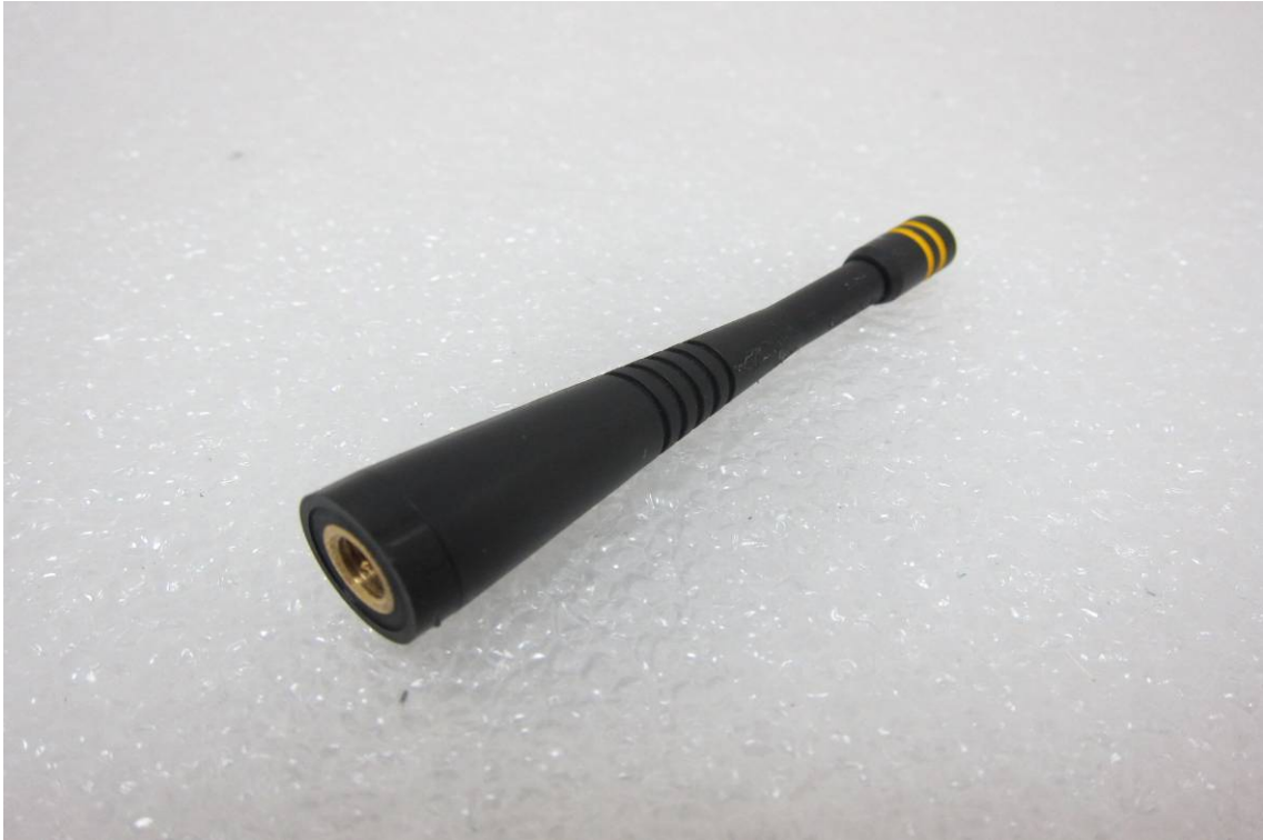
EUT – 4 (Rubber Antenna, P/N: ANT-916-CW-QW)
