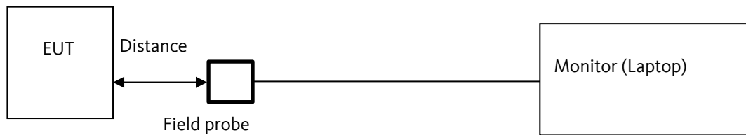
SETUP B (distance from surface of EUT to surface of probe) SCHEMATIC TEST SETUP OF FIELD STRENGTH MEASUREMENT
