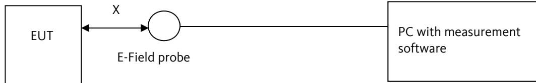
SCHEMATIC TEST SETUP OF ELECTRICAL FIELD STRENGTH MEASUREMENT ACC. TO SPR-002 [2]
