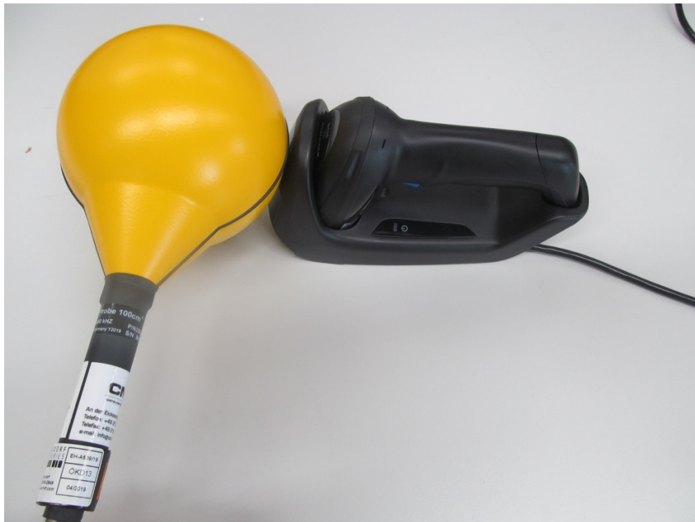
Exemplary photograph A1-3: RF E-field strength measurement (distance 0 mm)
