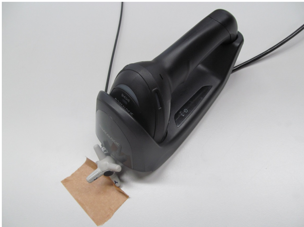
Exemplary photograph A1-4: RF H-field strength measurement (distance 0 mm)
