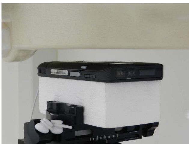
Back with Headset, Test Separation 15 mm
