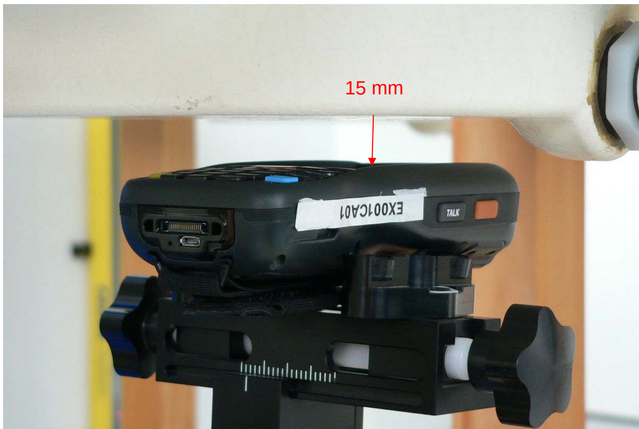
Fig. 60: Bottom view of body worn, display up (towards the phantom).
