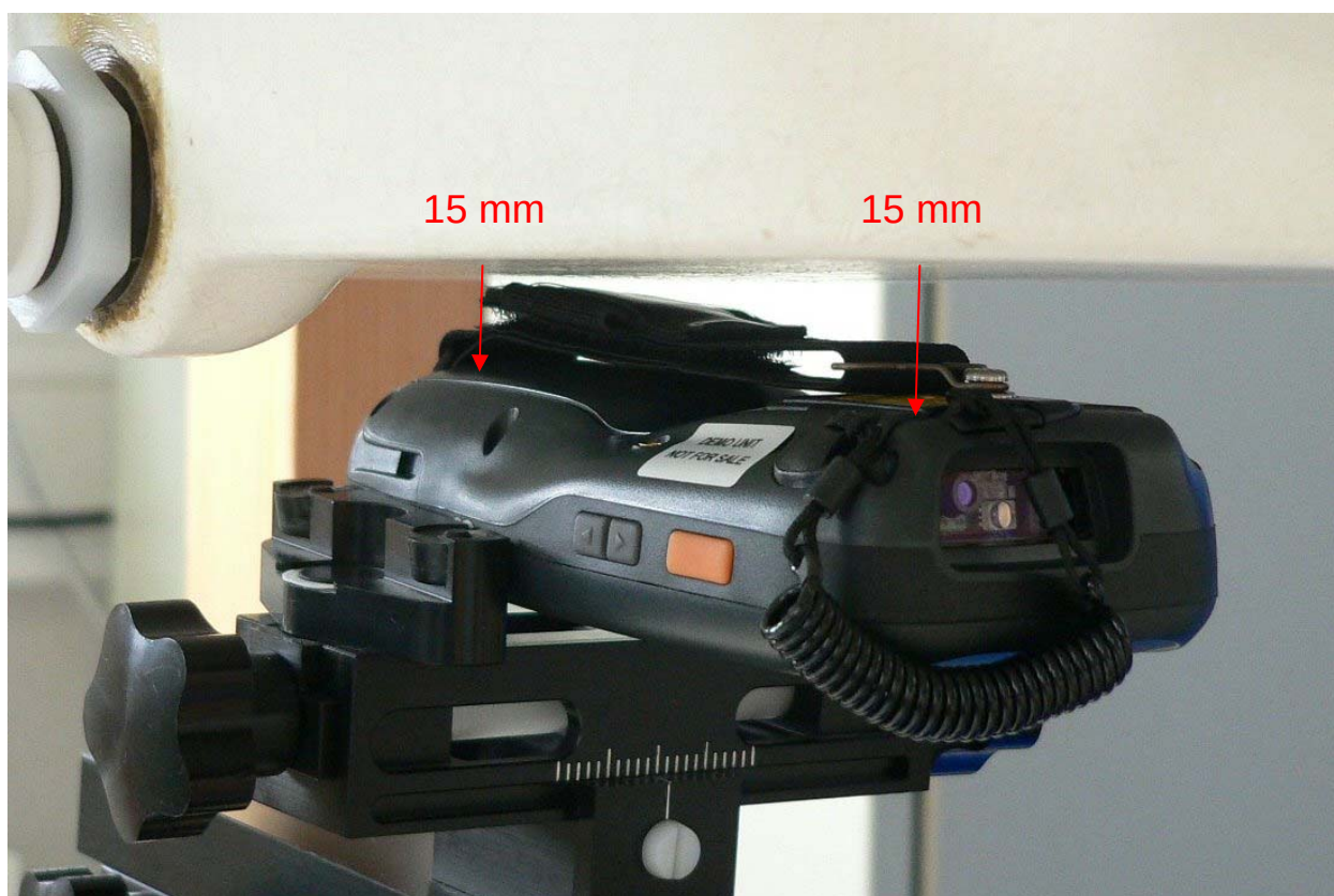
Fig. 63: Top view of body worn, display down (towards the ground).
