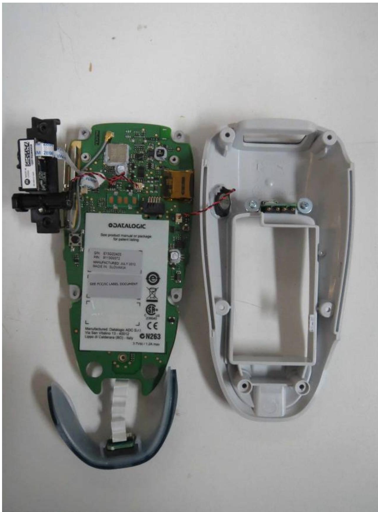
MAIN BOARD REAR VIEW
